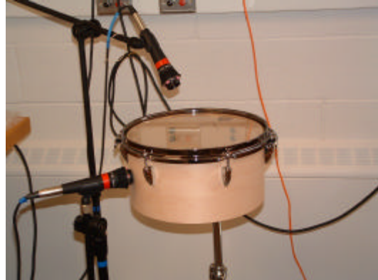
Fig. 3. Two microphone setup used to record drum sounds. One microphone will record overall drum sound, while the other will focus on the drum shell.
