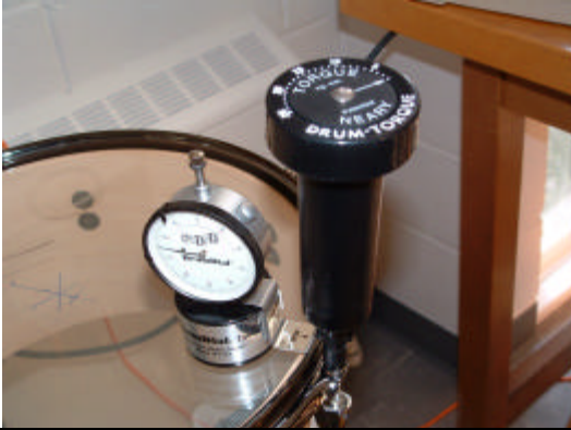
Fig. 4. Drum Dial and Drum Torque are used to make measurements for drum tuning.
